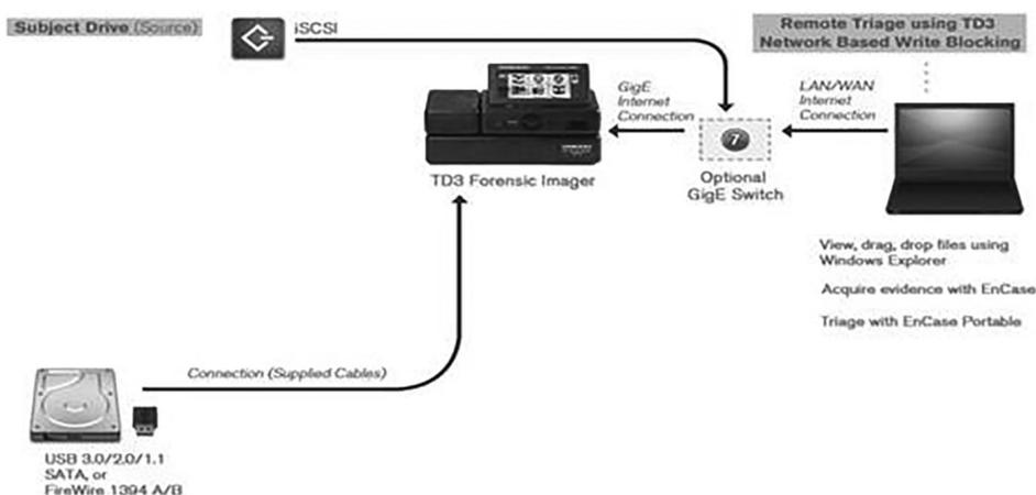
**Figure 1:** TD3 or TX1 device Triage/Collect action [23], operating in a role of the network write blocker, picture is provided by courtesy of GuidanceSoftware.
